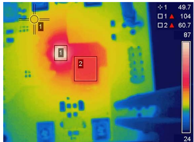
Figure 22: Thermal Image at V_{IN} = 19V , I_{OUT} = 12A (IR3476: 104^\circ C , Inductor: 61^\circ C , PCB: 50^\circ C )
